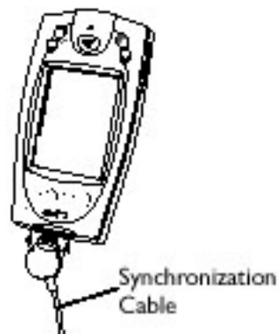
Figure 1-8: Connecting Cable to PPT 2700
