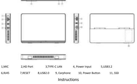
1. Connect the device with the display device (such as TV, screen, projector, etc.) via HD line, and select the "video input source" of the display device to the connected HD input channel. 2. Power supply: Connect the TYPE-C interface of the power cord of the accessories to the device and
