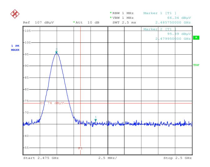
Comment: Band-edge test at high channel Comment: Peak detector F1=2483.5 MHz
