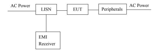
The EUT are connected to the main power through a line impedance stabilization network (LISN). This provides a 50 ohm/50uH coupling impedance for the measuring equipment. The peripheral devices are also connected to the main power through a LISN that provides a 50ohm/50uH coupling impedance with 50ohm termination.
