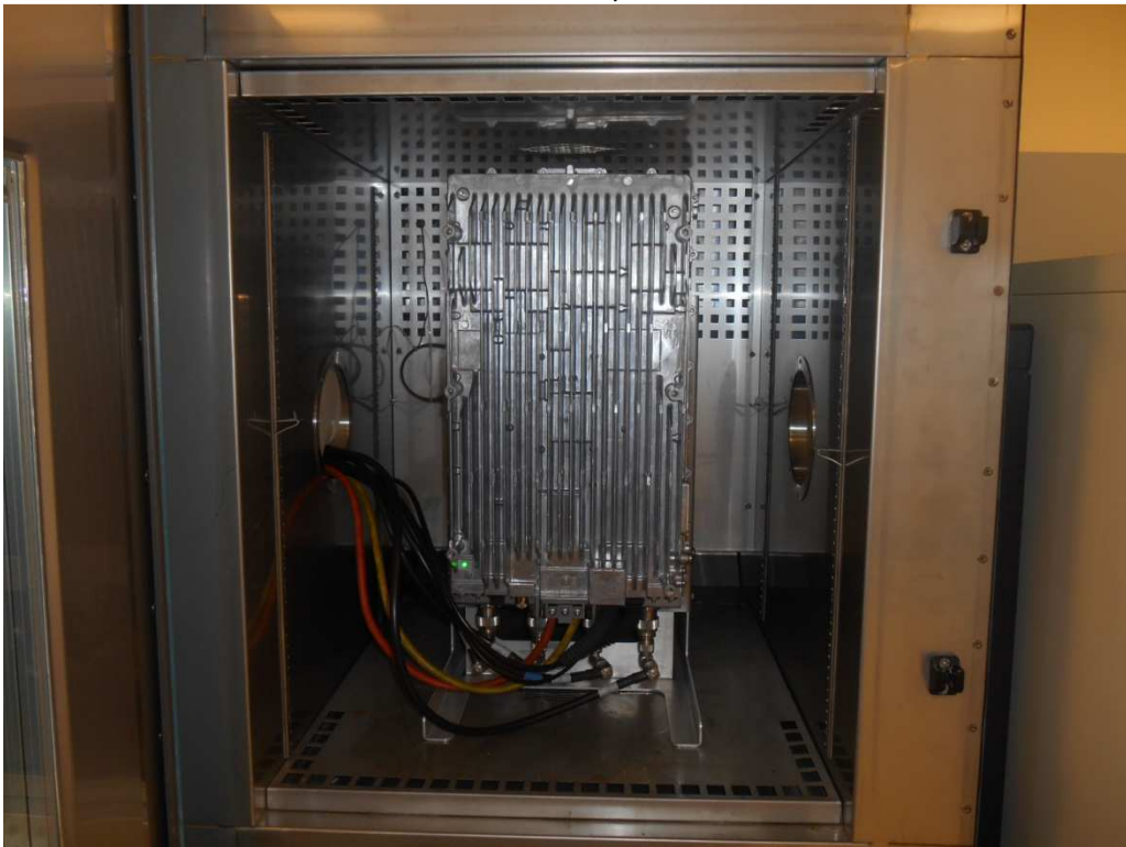
Frequency Stability Setup
