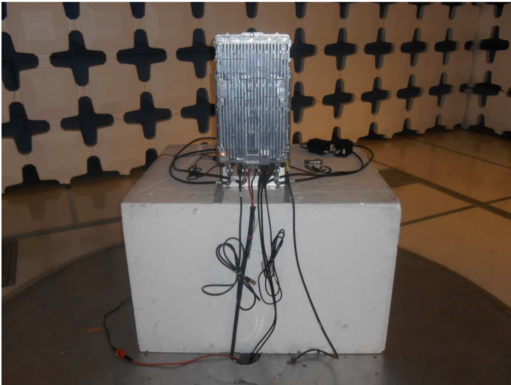
Radiated Emissions Setup - Front
