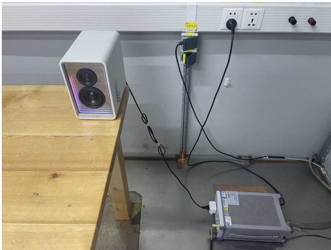
Photograph 2: Set-up for Radiated Spurious Emission, 30MHz - 1GHz
