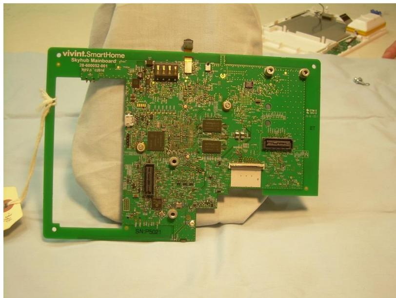
**2. Internal View Back Main PCB With Modules Removed**
