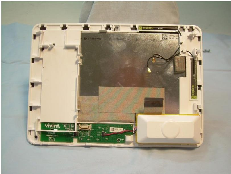
**6. Internal View Main PCB and Modules Removed (Metal Showing Is the Back of The LCD Screen – No Electronics Under the Back of LCD Screen)**
