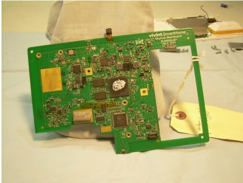
**5. Internal View Front Main PCB with Conductive Tape Removed**
