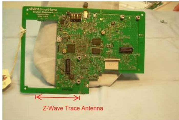
Photograph 12 – View of the Back Side of the Main PCB with Modules Removed
