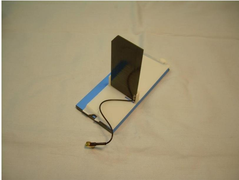
**7. Internal View of the Cell Antenna and Battery**
