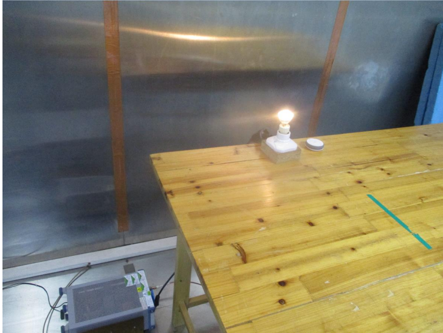
Photograph 2: Set-up for measurement of radiated emission
