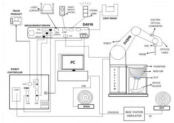
The DASY6 system for performing compliance tests consists of the following items:
