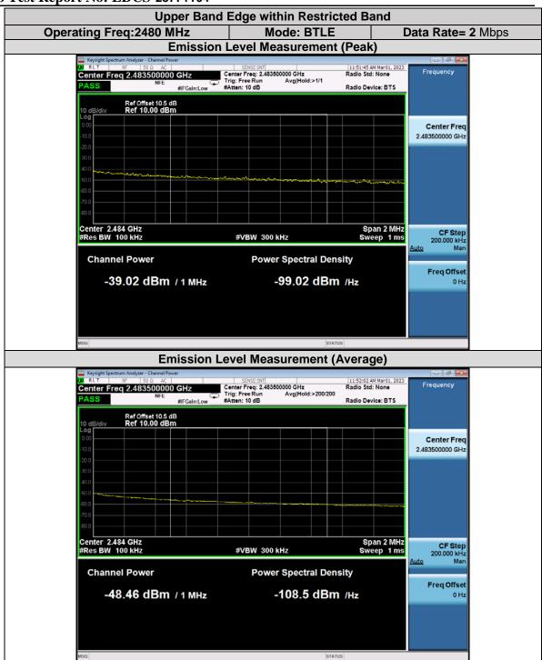
Note: Upper bandedge power integration was performed with the integration band centered on the bandedge instead of starting from the bandedge. As this results in a measurement being performed closer to the fundamental with higher amplitude, worst-case compliance is shown.
