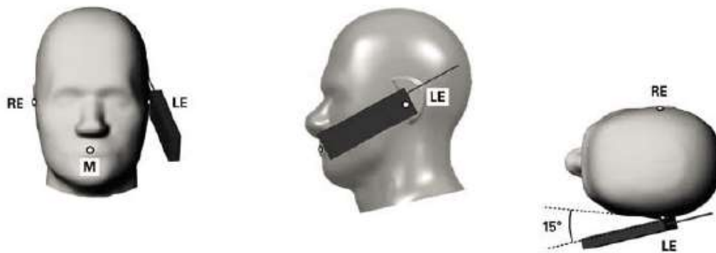
Fig.11.4 Illustration for Tilted Position
