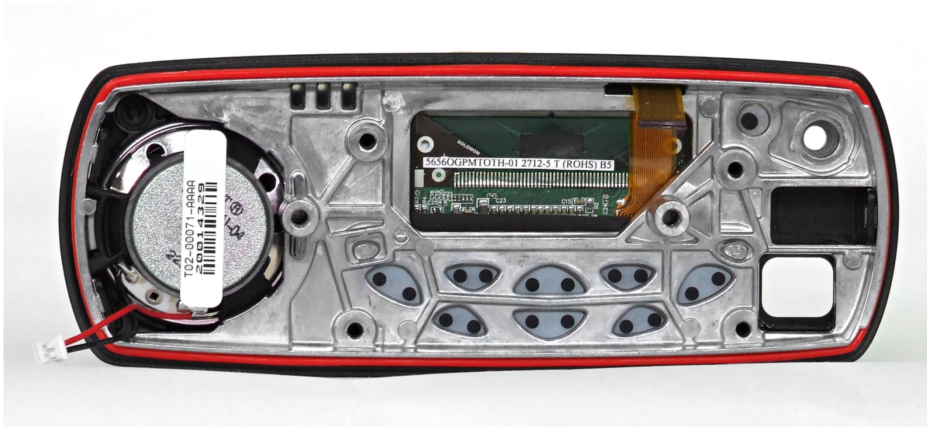
Photograph 06: Control Head – Internal with main PCB removed
