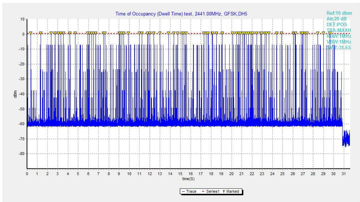
Fig.69. Number of Transmissions Measurement: Channel 39,Packet DH5
