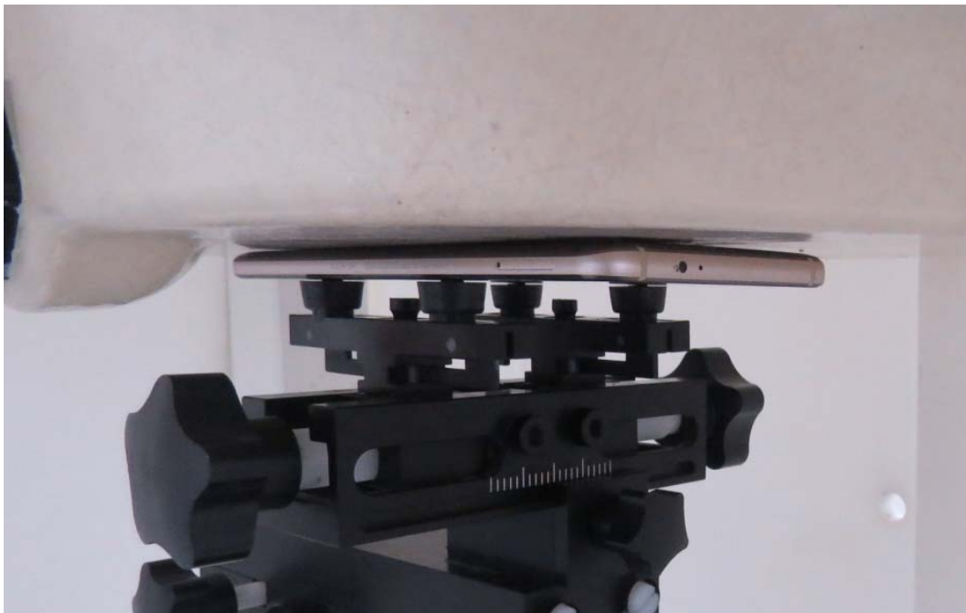
Picture 16: Back Side, the distance from handset to the bottom of the Phantom is 0mm
