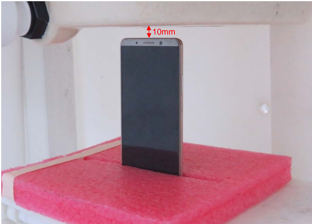
Picture 11: Top Side, the distance from handset to the bottom of the Phantom is 10mm
