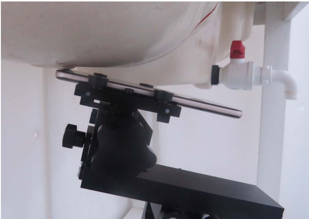
Picture 4: Right Hand Tilt 15 Degree Position
