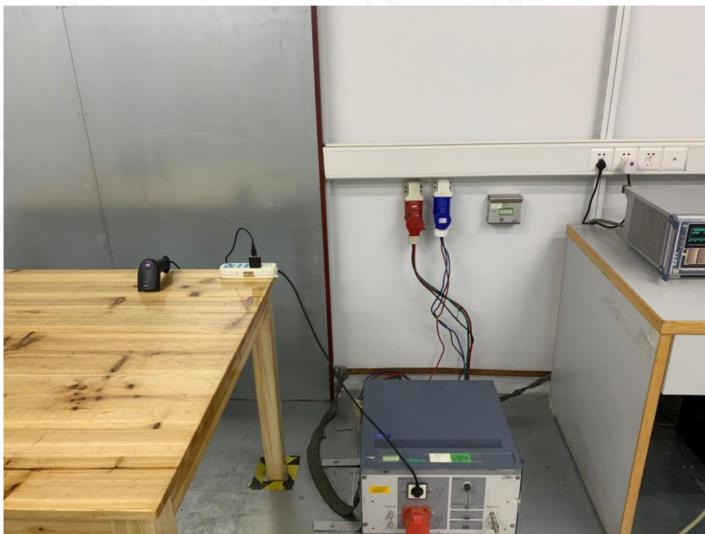
FCC RADIATED EMISSION TEST SETUP BELOW 1GHZ
