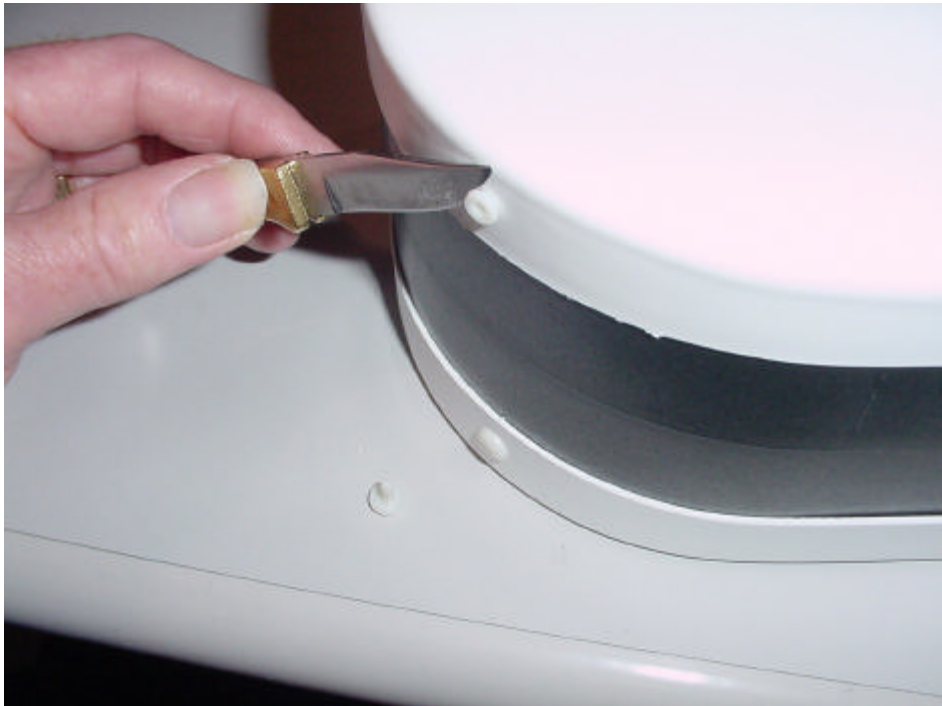
Figure C-2. Plastic Rivet Expansion Sleeve Removal
