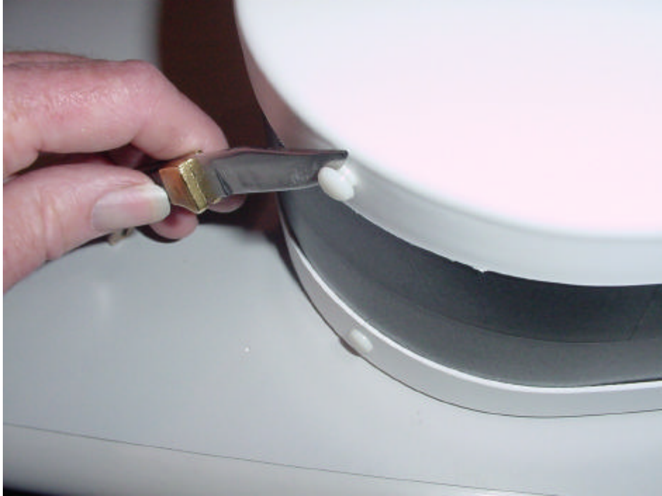
Figure C-1. Plastic Rivet Staking Pin Removal
