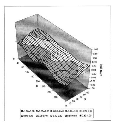
Spherical Isotropy Error < ± 0.4 dB
