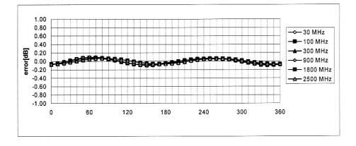
Axial Isotropy Error < ± 0.2 dB
