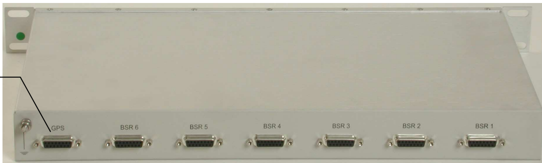
Figure 6-2: BSDU rear panel showing GPS port
