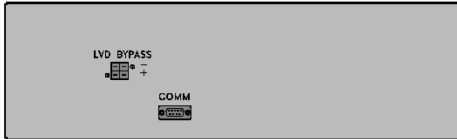
Figure 7-12: DC Distribution Rack rear view
