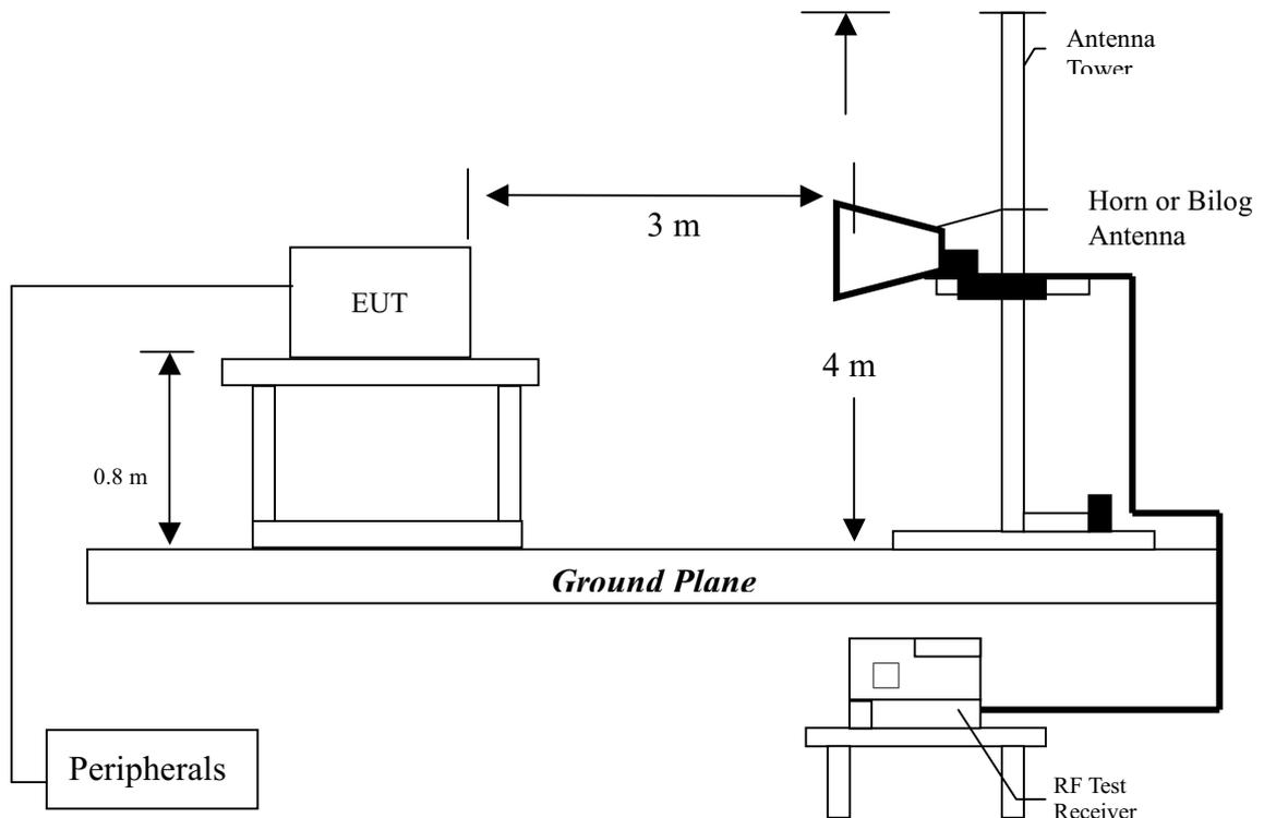
Radiated emission measurements were performed from 30MHz to 25GHz. Spectrum Analyzer Resolution Bandwidth is 100kHz or greater for frequencies 30MHz to 1GHz, 1MHz – for frequencies above 1GHz.
