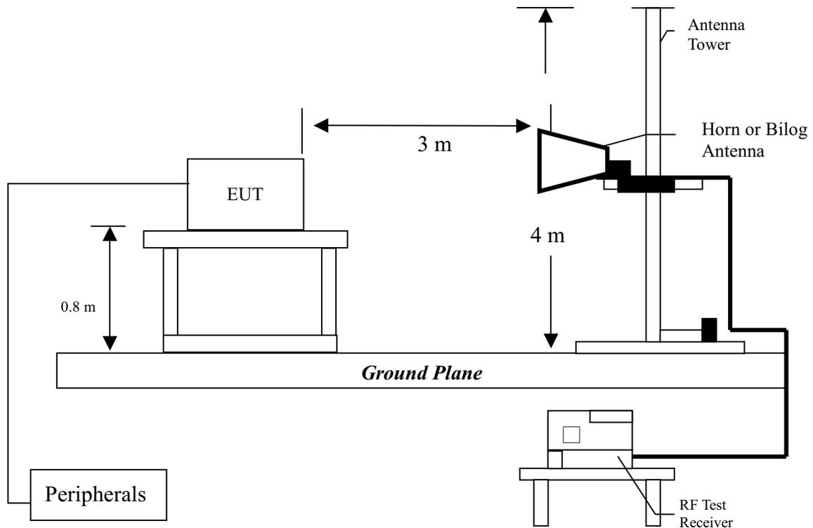
Radiated emission measurements were performed from 30MHz to tenth harmonic or 40GHz.
