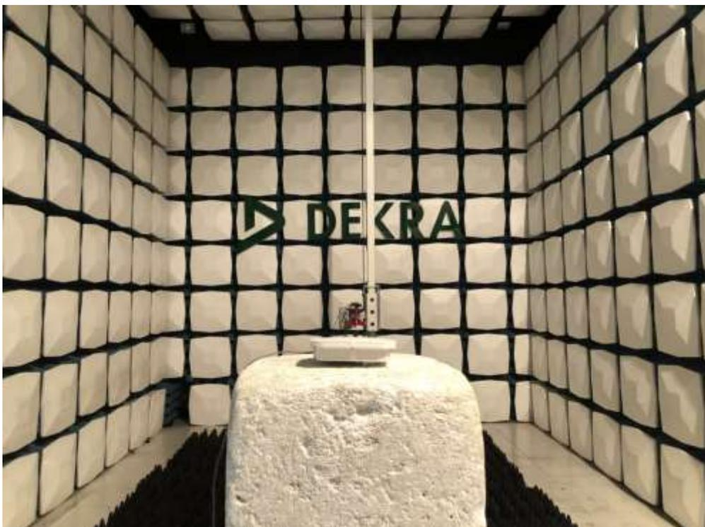
Description: Radiated Emission Test Setup for Above 18GHz(AP460C)
