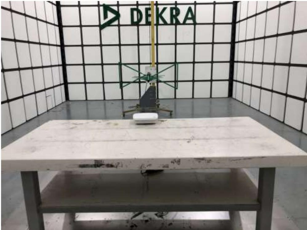
Description: Radiated Emission Test Setup for 1~18GHz(AP460C)
