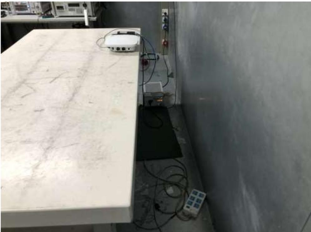
Description: Radiated Emission Test Setup for Below 1GHz(AP460C)
