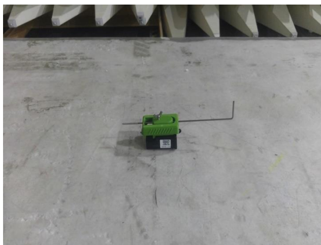
Photograph 8.1.3 Setup for final radiated emission measurements, EUT cabling
