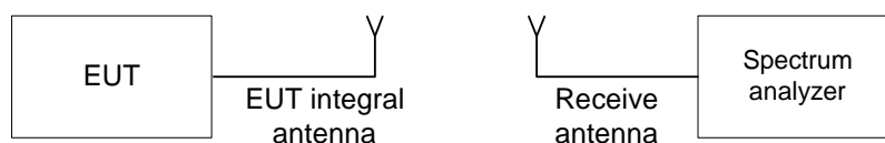
Figure 7.1.1 Setup for transmitter shut down test
