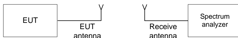
Figure 7.4.1 Occupied bandwidth test setup
