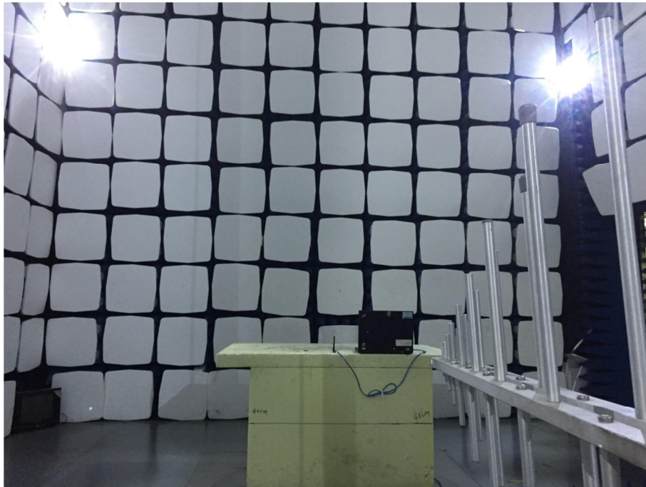
Radiation Emission Test Setup (30MHz to 1GHz)
