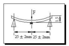
Welded the product in the middle of the PCB board of  $1.6\pm0.2$ mm according to the drawing, apply the force by the arrow direction: 1mm / S, bending distance: 1.5mm, keep  $5\pm1$ S, the product metal layer does not fall off. Weld the product to the center part of the PCB with the thickness  $1.6\pm0.2$ mm as the illustration shows , and keep exerting force arrow-ward on it at speed of :1mm/S , and hold for  $5\pm1$ S at the position of 1.5mm bending distance , so far , any peeling off of the
