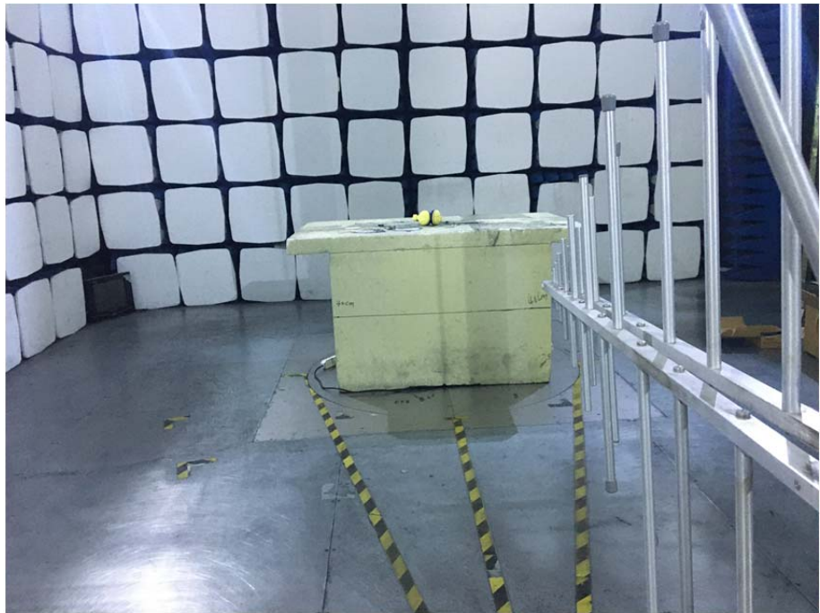
Radiation Emission Test Setup (30MHz to 1GHz)
