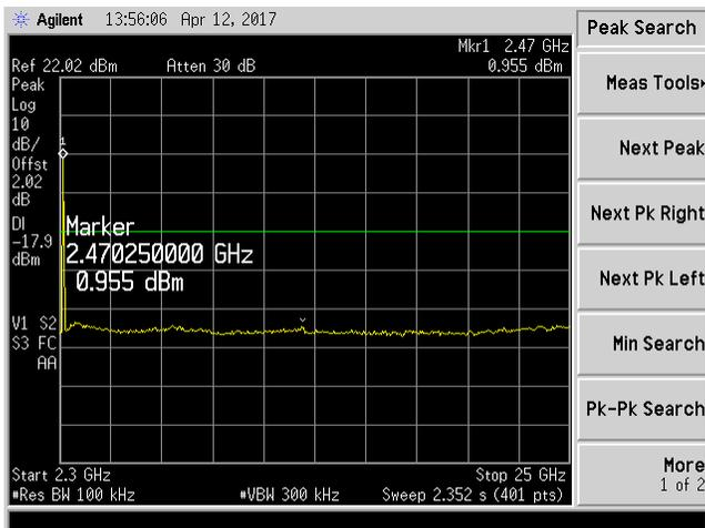
High Channel 2480 MHz Conducted Spurious emissions (30 MHz – 25 GHz)
