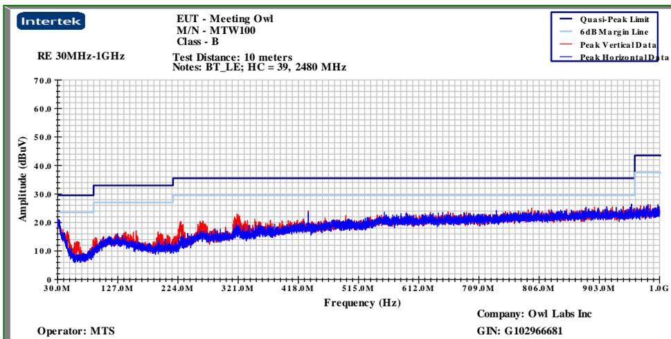
**30-1000 MHz Transmitter Spurious Emissions (Worst Case data – Mid Channel: 2442 MHz)**
