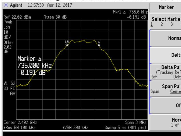
6dB Bandwidth @ Mid Channel 2442 MHz = 735.0 kHz
