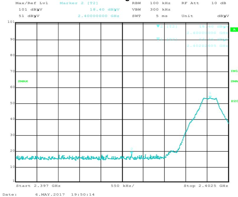
Emissions at lower band edge are 20 dB lower than the fundamental.
