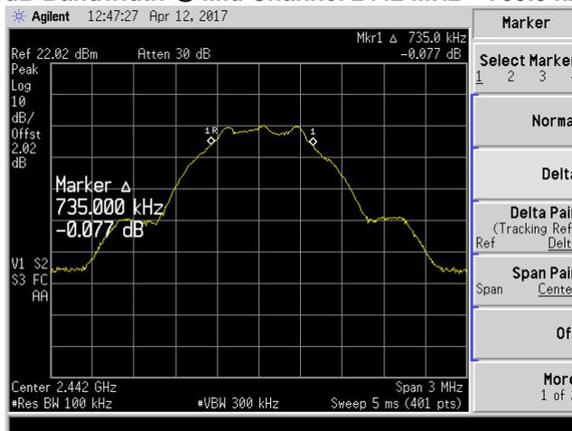
6dB Bandwidth @ High Channel 2480 MHz = 735.0 kHz
