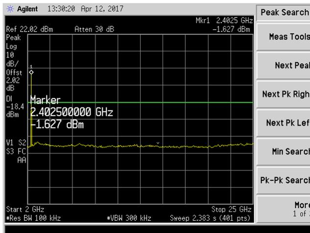
Mid Channel 2442 MHz Conducted Spurious emissions (30 MHz – 25 GHz)
