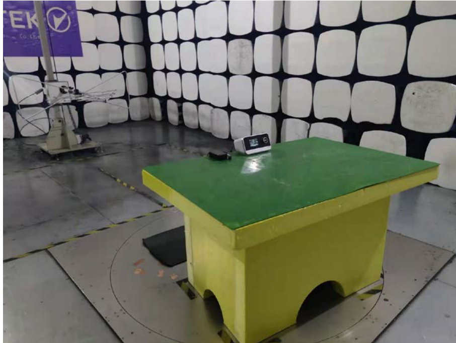
Spurious Emission Test Setup (Above 1GHz)
