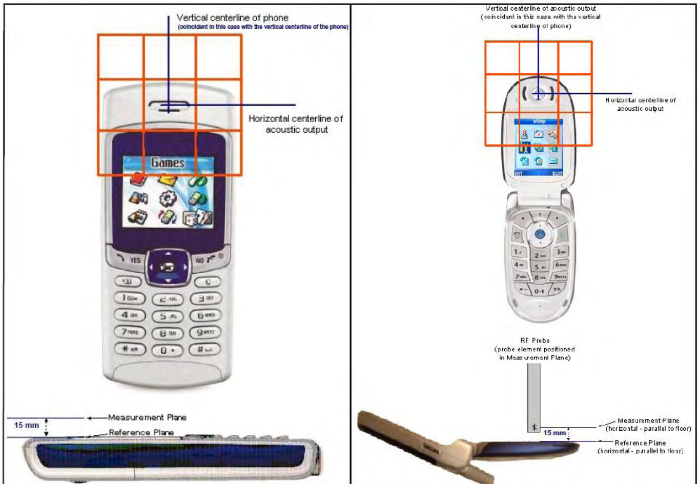
Fig-3.4 EUT Reference and Plane
