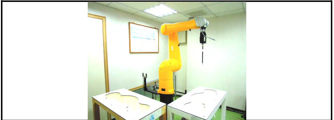
Fig-3.2 DASY5 Measurement System
