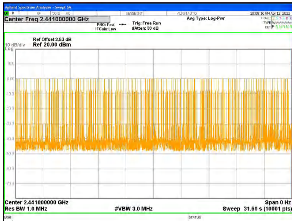
Dwell NVNT 1-DH5 2441MHz Ant1 One Burst
