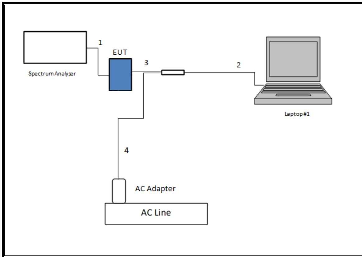
**DIAGRAM FOR RADIATED AND LINE CONDUCTED EMISSIONS TESTS**
