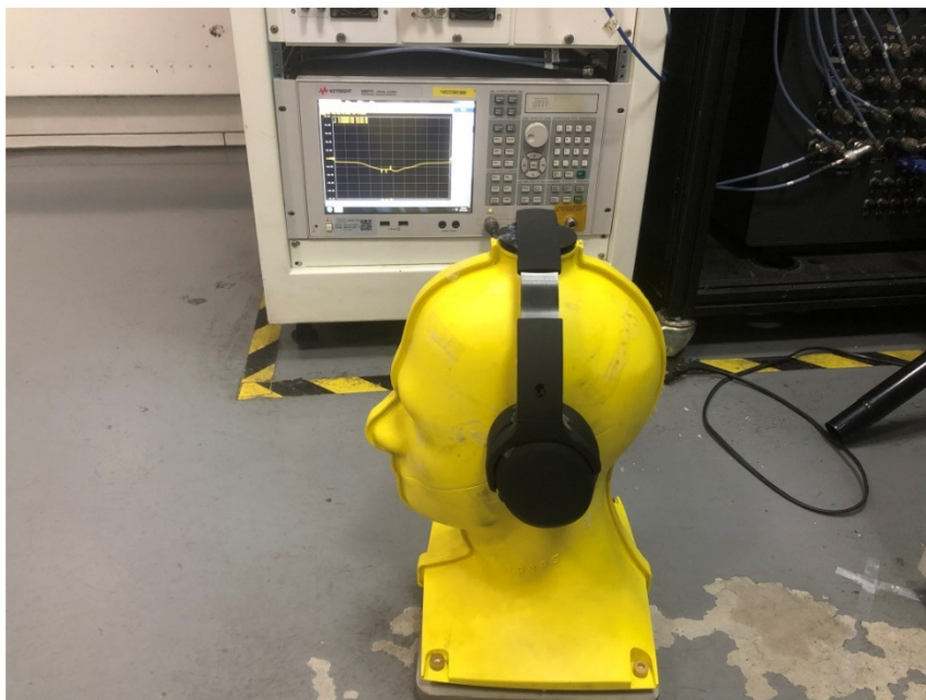
Beside Head #2 Impedance Setup
