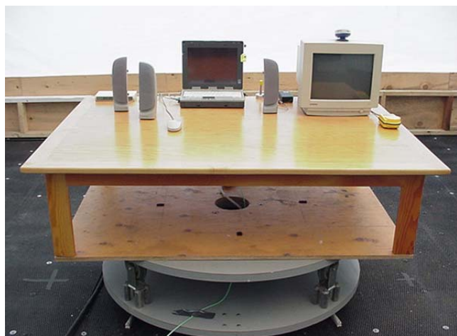
Photograph E.7-3 - Front of Radiated Emission Setup
