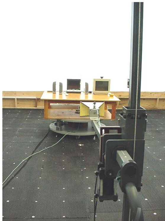
Photograph E.7-2 - Vertical Horn Receive Antenna with DUT
