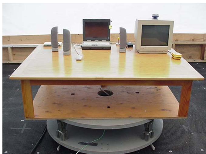
Photograph C.7-2 - Front of Radiated Emission Setup
