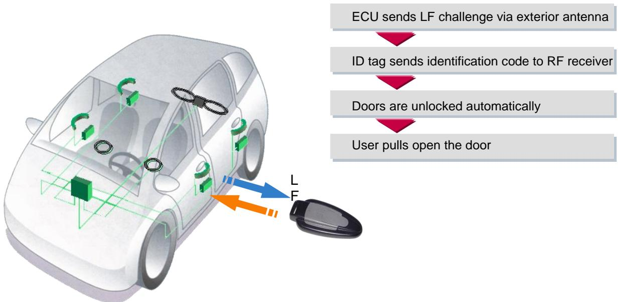
**Figure 1: Principle of Communication**
