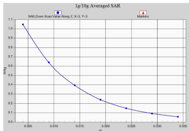
Fig.A.1- 6 Z-Scan at power reference point (W1900)
