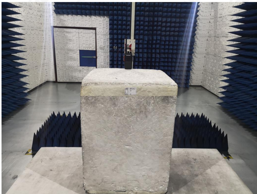
RADIATED EMISSION ABOVE 1G TEST SETUP
