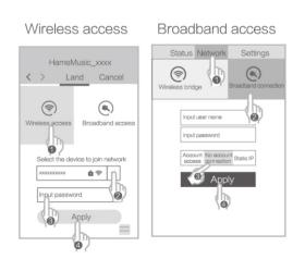
Note: Success of wireless bridge will prompt that "The mobile phone and device has been disconnected in the system settings, please reconnect the WIFI to the Internet. " Success of broadband connection will display the state connection information and IP information.
