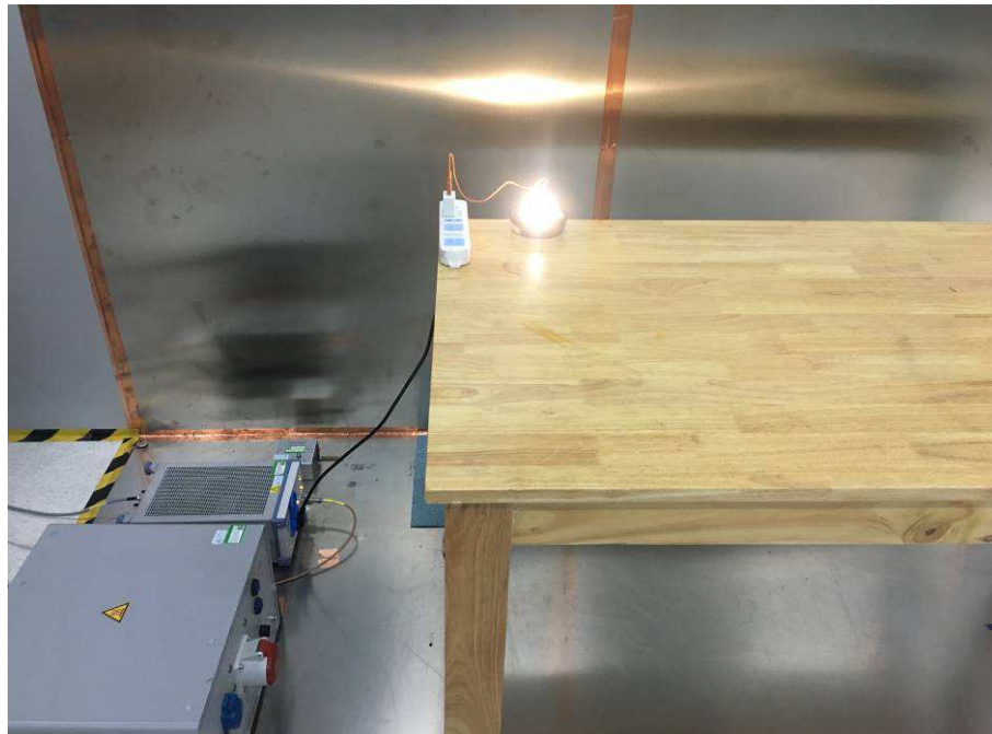
Photograph 4: Set-up for Conducted Emission on AC Mains
