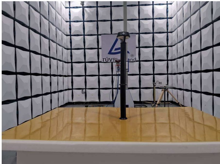
Photograph 3: Set-up for Radiated Spurious Emission, 1GHz - 18GHz
