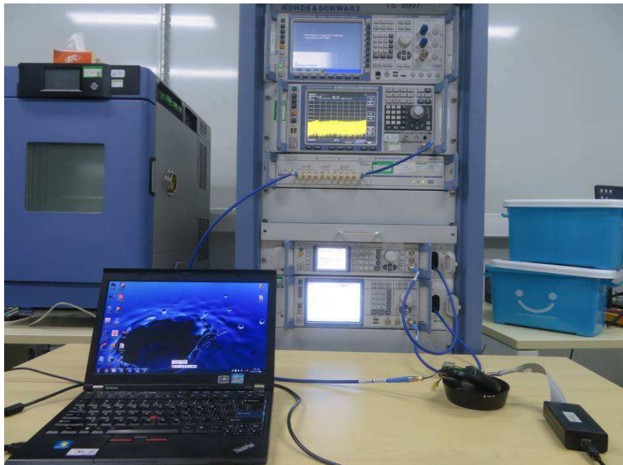
Photograph 1: Set-up for Radio Spectrum Test
