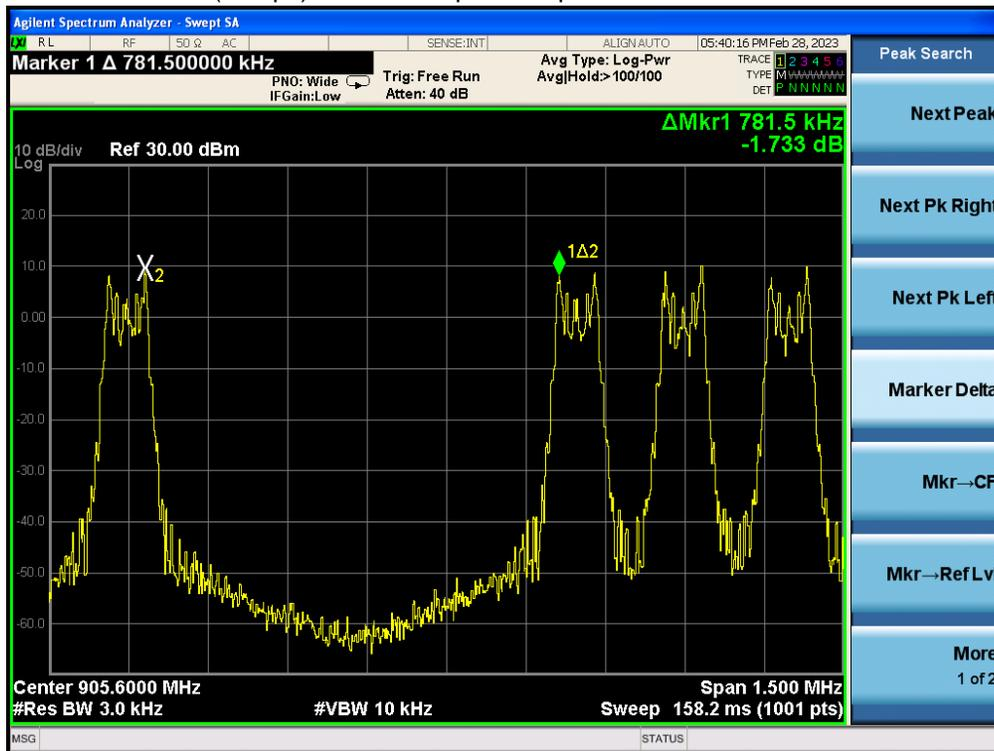
(1Mbps) Channel Separation plot on channel 52-53
