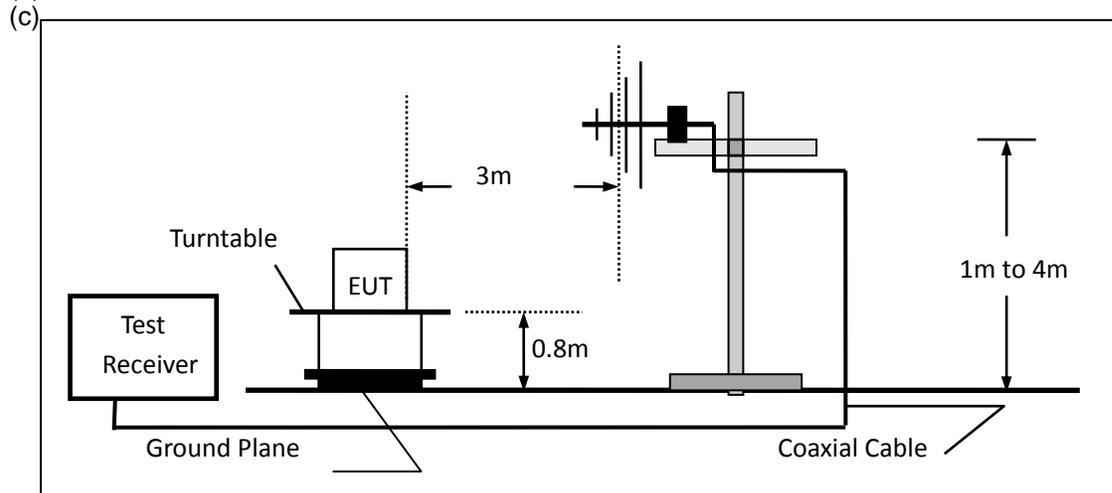
(c) For radiated emissions above 1000MHz
