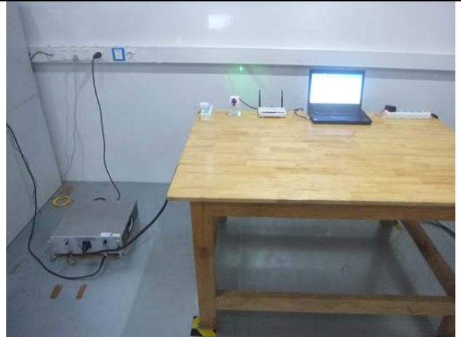
Conducted Emissions Test Setup Side View
