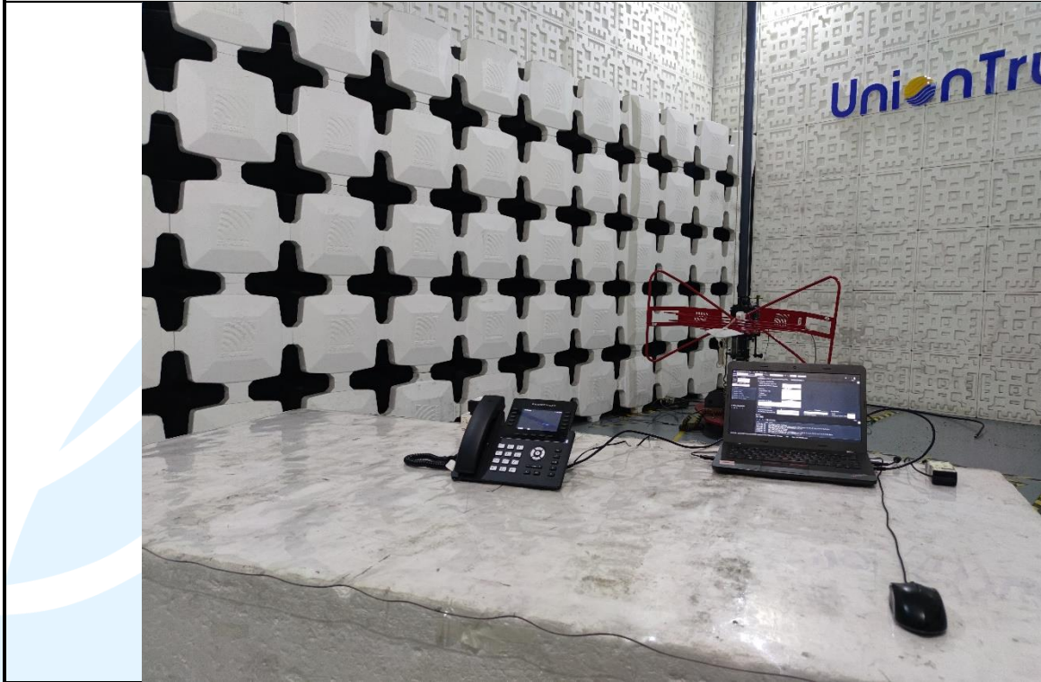
Radiated emission Test Setup (30 MHz~1 GHz)
