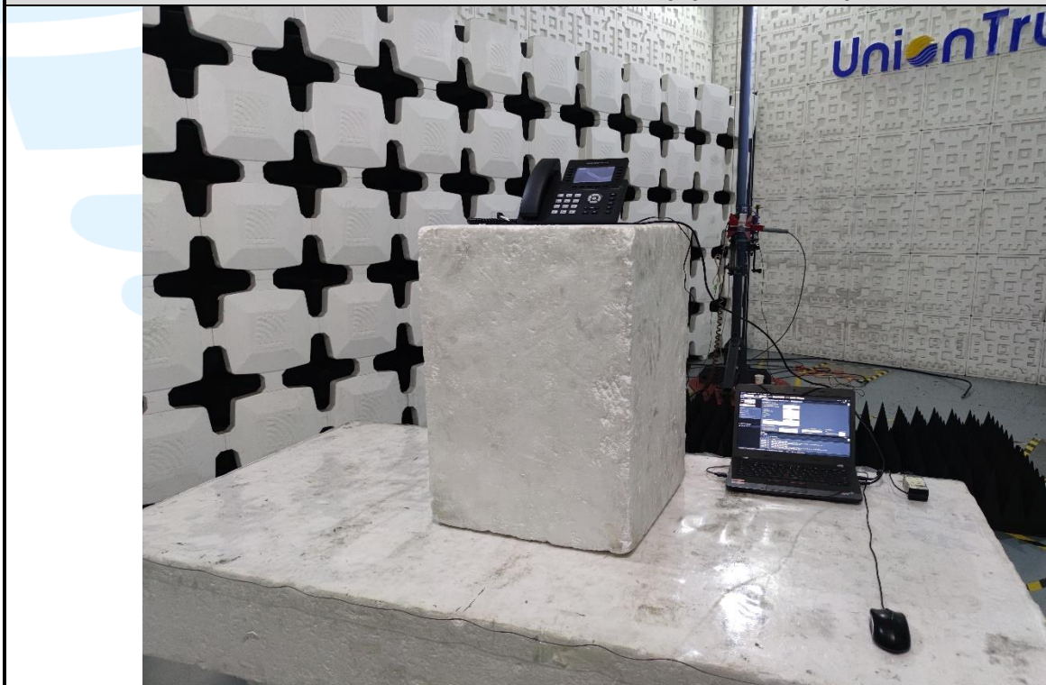
Radiated emission Test Setup (Above 1 GHz)
