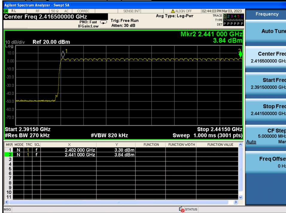
**Number of Hopping Channels 2(FH)      Hopping mode : Enable & 8DPSK**
