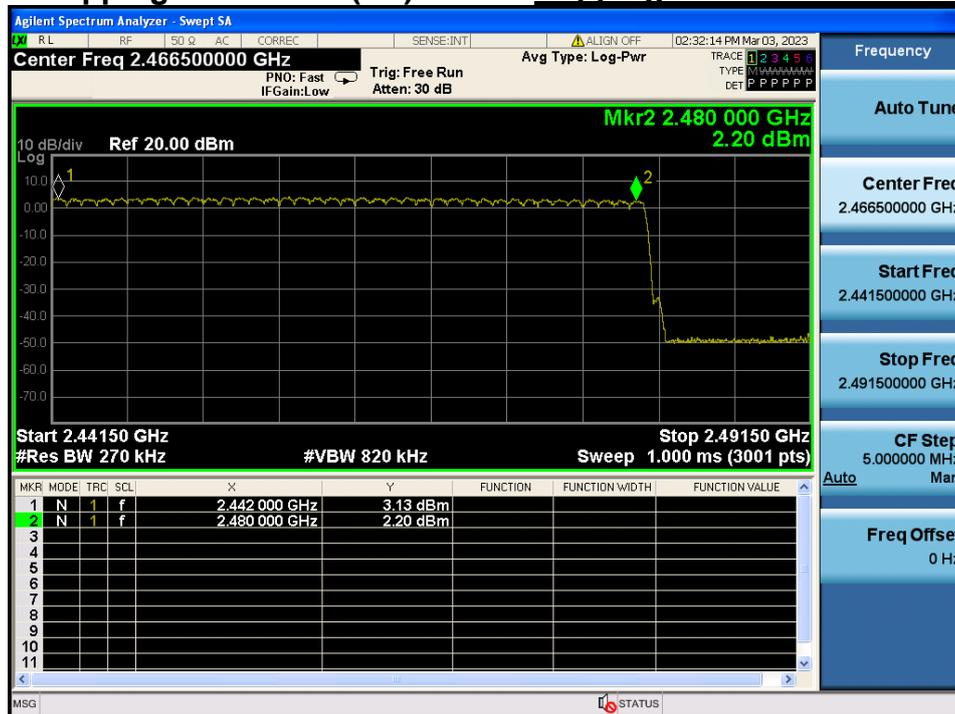
**Number of Hopping Channels 1(FH)      Hopping mode : Enable&8DPSK**
