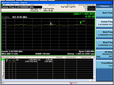
Carrier Frequency Separation (AFH) <u>Hopping mode : Enable&8DPSK</u>
