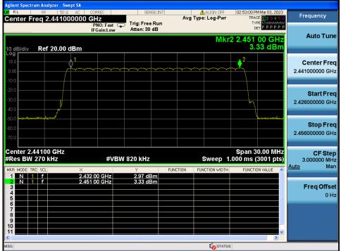
Number of Hopping Channels 1(AFH) <u>Hopping mode : Enable & 8DPSK</u>
