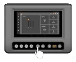
Figure 36: Press EXT to wake the display
