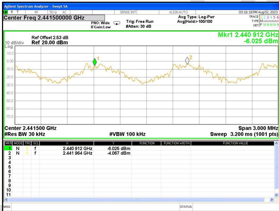
CFS NVNT 2-DH1 2441MHz Ant1
