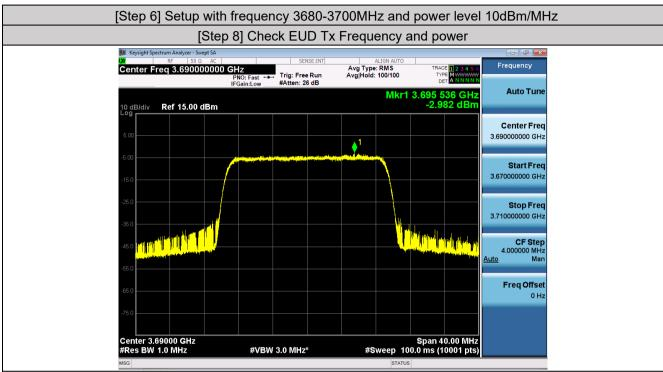
EIRP PSD=-2.982+3.4+4.5+3=7.918dBm/MHz, Antenna gain is 3.4dBi,the path loss is 4.5dB, the MIMO Factor is 3dB
