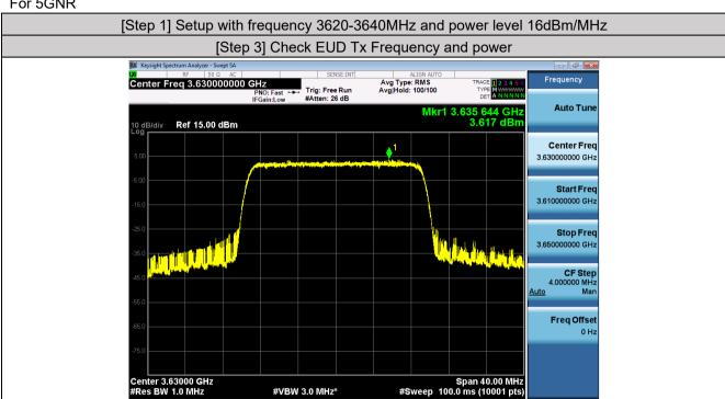
EIRP PSD=3.617+3.4+4.5+3=14.517dBm/MHz, Antenna gain is 3.4dBi, the path loss is 4.5dB, the MIMO Factor is 3dB
