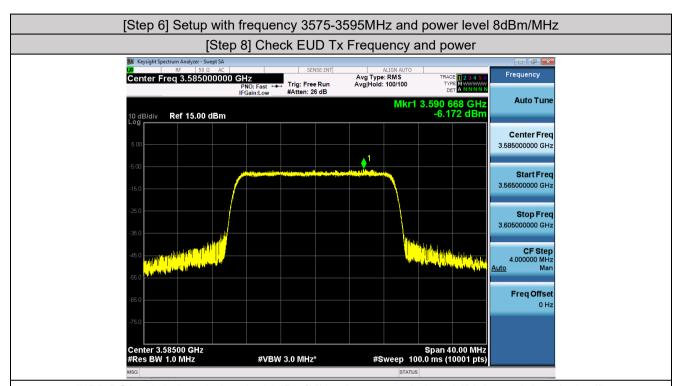
EIRP PSD=-6.172+3.4+4.5=1.728dBm/MHz, Antenna gain is 3.4dBi,the path loss is 4.5dB
