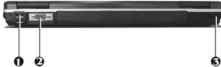
1. USB 2.0 Ports 2. VGA Port 3. Kensington Lock Hole
