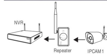
Note: To use a wireless repeater, the repeater must first be paired to the wireless NVR. Press and hold the wireless repeater for 10 seconds. When the NVR status light flashes quickly, it will automatically pair with the NVR without any sense when approaching the wireless NVR. After successful pairing, the NVR status light is always on.
