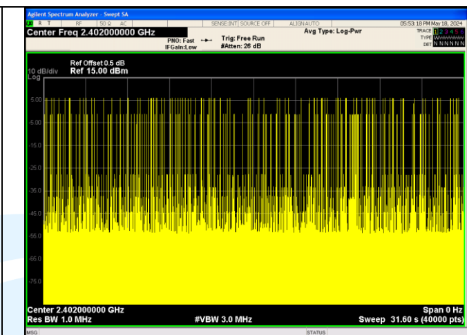
Number of Pulses in 31.6 seconds 8DPSK_3-DH5
