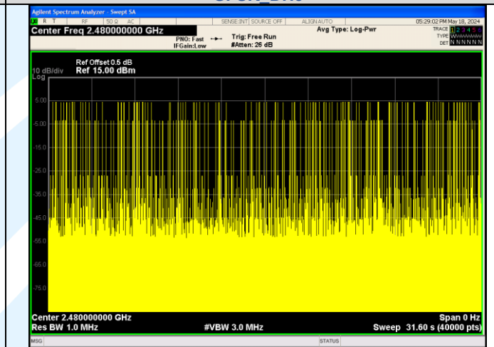
Number of Pulses in 31.6 seconds GFSK DH5
