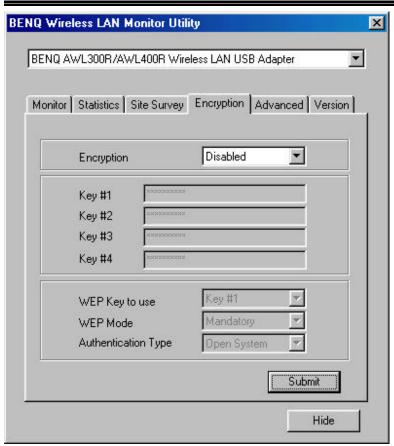
According to WEP function select, this panel allows the entry of 64-bit encryption and 128-bit key. Each key must consist of hex digits to be written to the driver and registry. This means that only digit 0-9 and letters A-F are valid entries. Therefore, if entered incorrectly, the program will not write keys to a driver.
