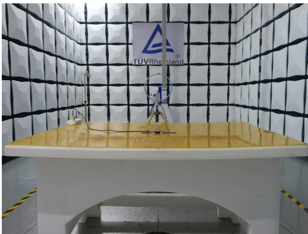
Photograph 1: Set-up for Radiated Spurious Emission, Below 30MHz
