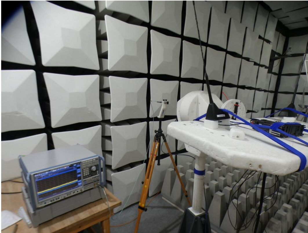
Photo 5: Test setup for radiated measurements, detailed view (26 - 40 GHz; Fully anechoic chamber, FCC Part 15.407; ANSI C63.10)
