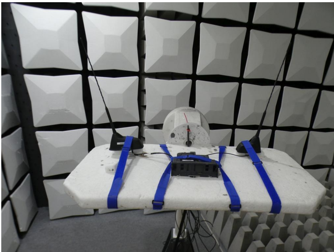
Photo 4: Test setup for radiated measurements, detailed view (1 - 26 GHz; Fully anechoic chamber, FCC Part 15.247, 15.407, 22, 24, 27 and 90; ANSI C63.10)
