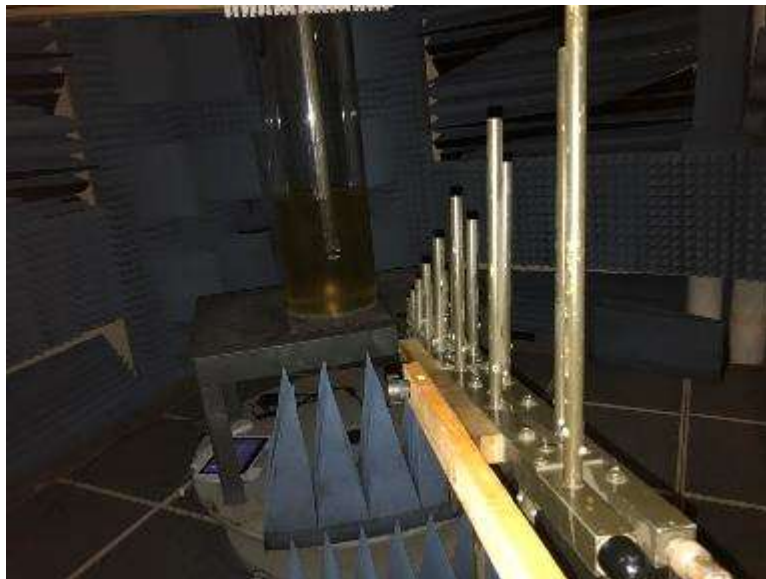
EUT Inside Torso Simulator for Loss Measurement
