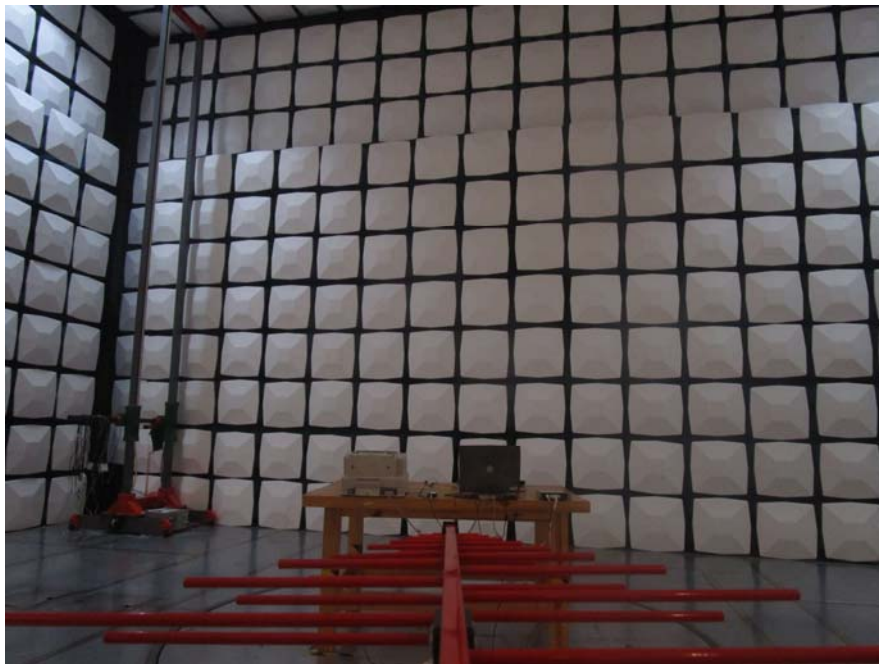
Radiated Emission Below 1GHz – Rear View
